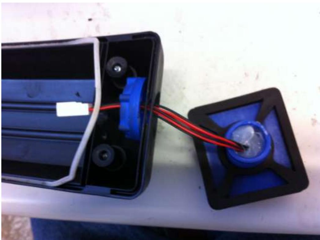
Tighten it up until the thick gasket is squashed down hard against the pendant.
