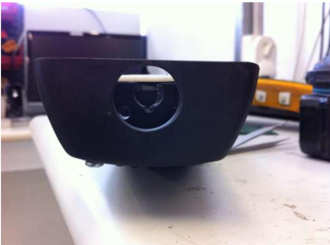
In this case the step drill used drill proceeded into the next plastic wall. We will use this hole to run the cables into the pendant.
