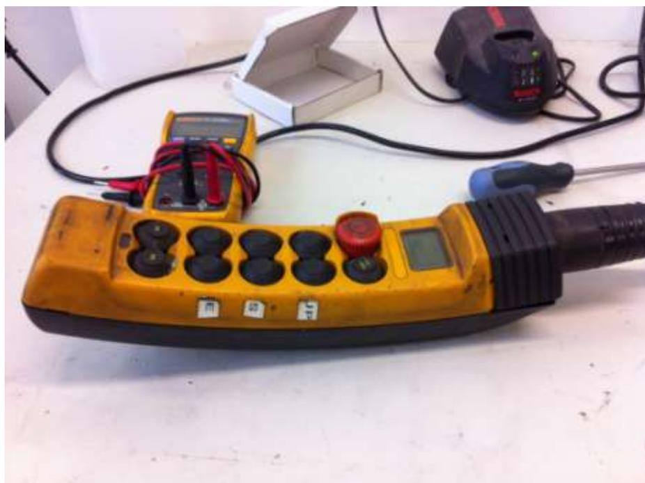
**Step 1:** Isolate the 48VAC going to the pendant. Undo the 4 case screws from the back of the pendant. Remove the back cover.
