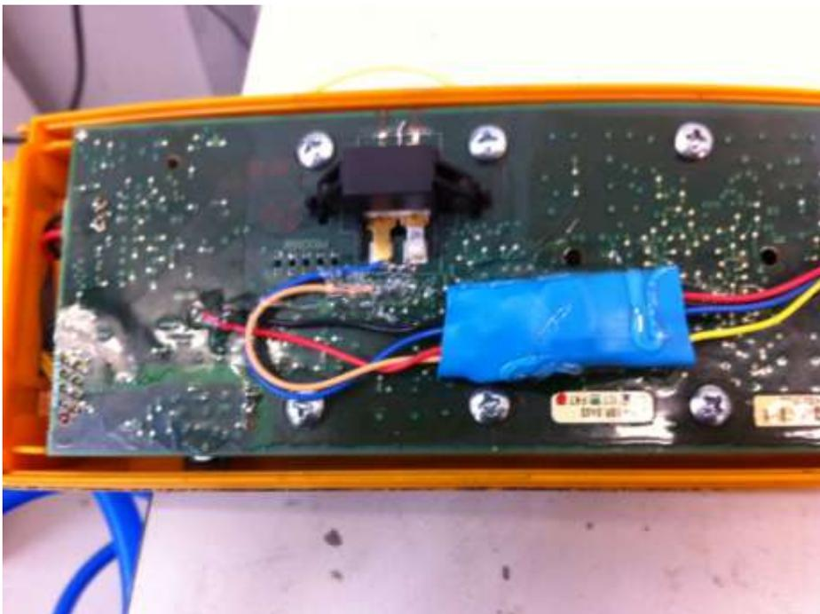
That completes the wiring install for the Pendant.
