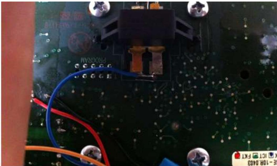
Its important that when you solder the blue wire across the two pads that it doesn't inhibit the contacts of the switch. A pointy tip soldering iron helps here.
