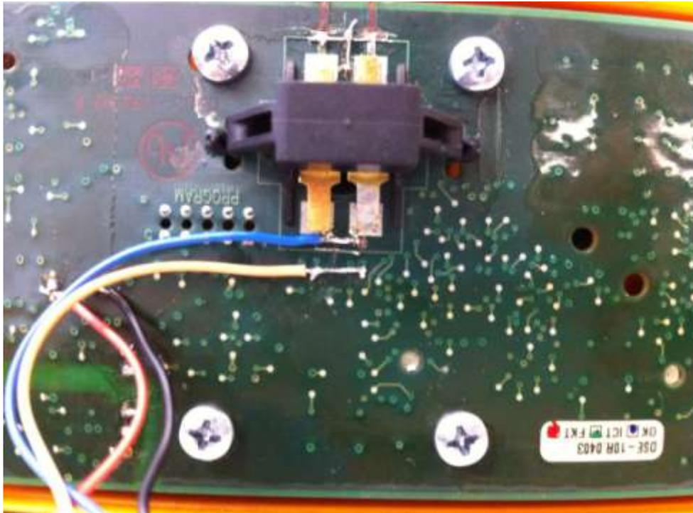
The orange wire goes to both the little test points just below the switch. These pads are very small, so once you have it soldered down put some sort of adhesive (eg neutral cure silicone, hotmelt glue) on the pcb to hold the wire in place and stress relieve it. It's a good idea to do this for all the wires.
